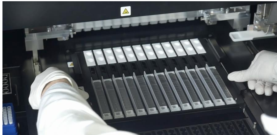
Figure 5-63: Loading Extraction cassette rack on the instrument.
